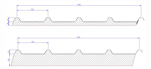
Figure 1: JI ECO PIR in thicknesses 30 mm & 100 mm
